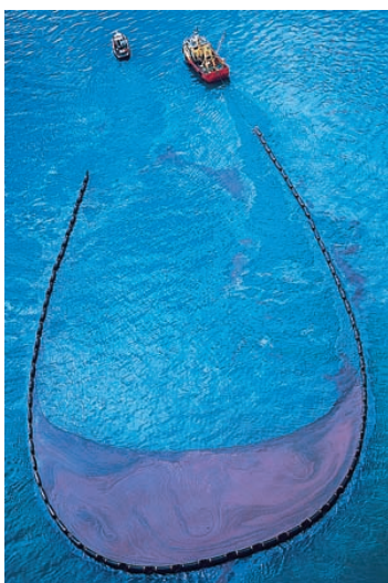
Figure 8.6 Oil spills can be contained to some extent by using trawlers and a boom apparatus because oil and water, having different polarities, are relatively insoluble in each other. The oil, which is of lower density, floats on top of the water.
